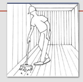
Upon the receipt of the container, a short internal inspection is necessary to find any existing sharp metallic particles on the internal walls, that could injure the technician and/or damage the liner, compromising the thermal insulation efficiency. If sharp metallic particles/provisions are found, use a hammer, pliers or other tools to smoothen or remove them.
