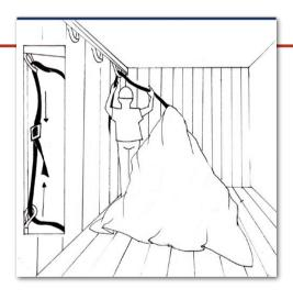
Insert the black lanyard in the first ring on the upper left corner and the other lanyard on the lower left corner. Tie both lanyards together using the rings of the upper lanyard.
