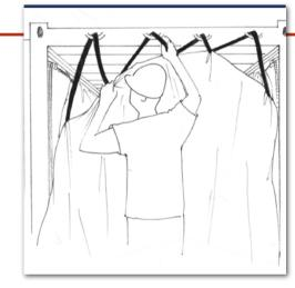
Fix the liner at the entrance door, on the external upper side of the container. Turn over the front side of the liner on the roof.
